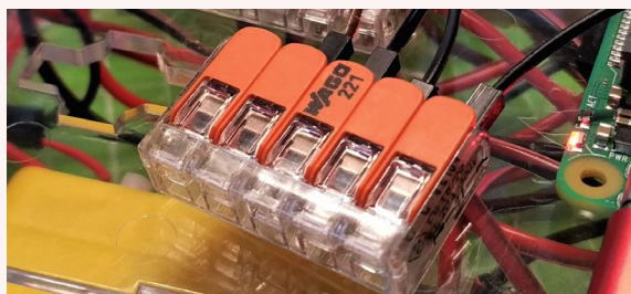
A Wago 221 connector can turn one connection into many. We used it to make a common ground reference and break out the 5V power.
